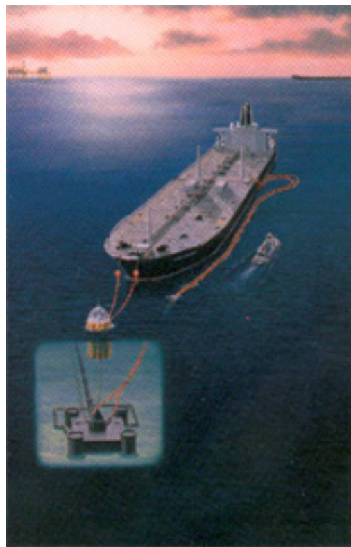
A ULCC tanker connected to a SALM berth with the LOOP terminal on the horizon
